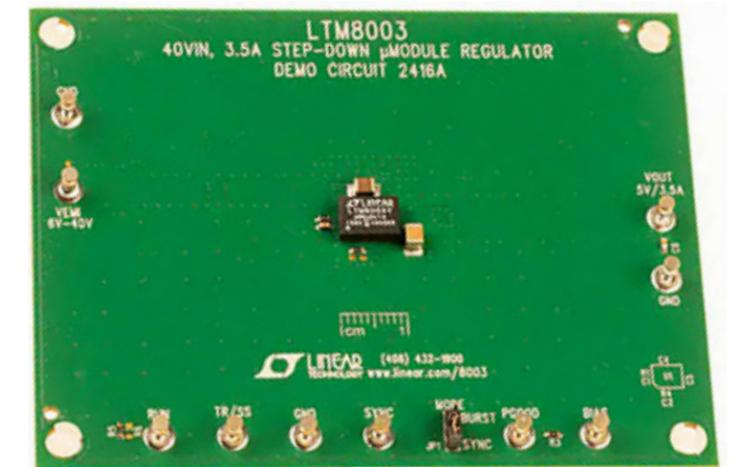
Figure 10: The DC2416A demo board simplifies connection with and evaluation of the LTM8003 Silent Switcher device. (Image source: Analog Devices)
