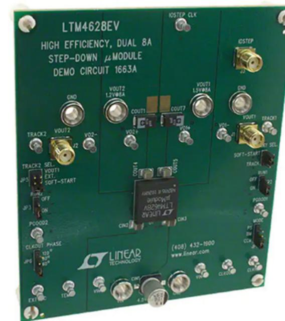
Figure 15: Evaluation of the single/dual-output LTM4628 is accelerated with the use of its DC1663A demo board. (Image source: Analog Devices)
