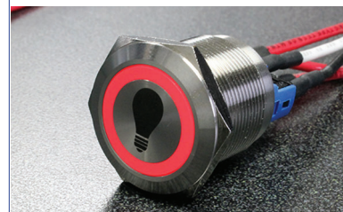
DH Series 22mm, 25mm, 28mm & 30mm IP67 Sealing Degree Momentary or Latching Panel Mount 2A@24VDC / 125VAC, 1A@250VAC
