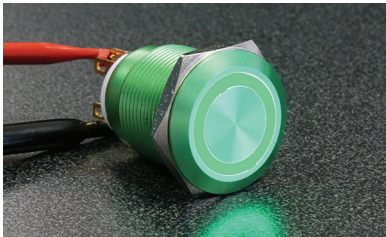
AH Series 19mm IP67 Sealing Degree Momentary Panel Mount 1A@24VDC / 125VAC, 0.5A@250VAC
