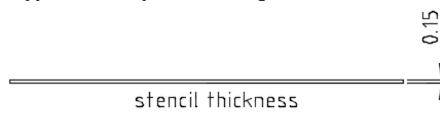
Figure 9: RECOMMENDED STENCIL THICKNESS REQUIRMENT (YOUR CONFIGURATION MAY VARY)
