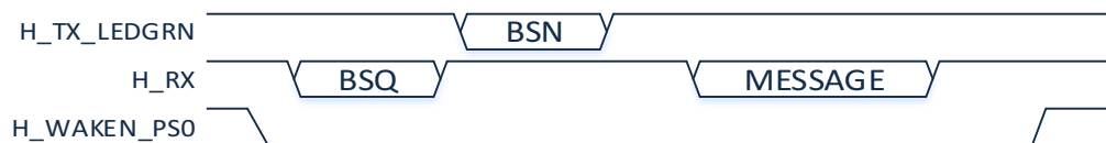
Figure 6: UART-SHTP - Sending a message to the FSP201
